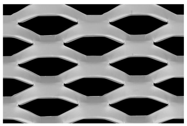
LW Pitch:76.20mmStrand Width:11.00mmSW Pitch:35.00mmThickness:3.00mmWeight:5.09 kg / m2Open Area:37%
